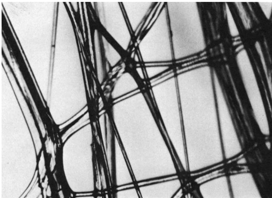
Fig. 3. Optical micrograph for PVA VTF fibers obtained winding on the second roller. The fibers were dried on the second roller.
